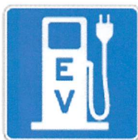
D9-11b Electric Vehicle Charging
